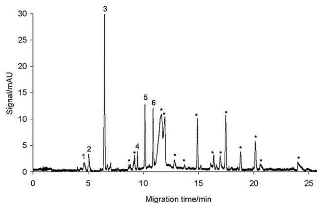
Fig. 5. Electropherogram at optimised running condition showing compounds produced for a decomposition fluid sample with identified peaks: tryptamine (1), tyramine (2), neutral (3), tryptophan (4), tyrosine (5), phenylalanine (6) and unidentified components (\*) [38].
