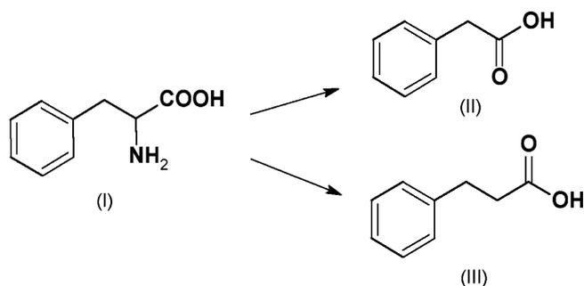
Fig. 3. Degradation pathway of phenylalanine to produce phenylacetic and phenylpropionic acids.
